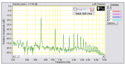
**Fig. 1(b).** Spectrum view at higher pressure with shifted frequency at the same tube length of 110 cm.
