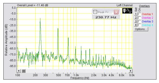
Fig. 1(a). Spectrum view of lip driven pipe of length of 110cm. & diameter 1.9cm.
